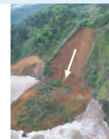
debris avalanche (unchanneled flow)
