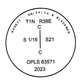
I used 14° East declination in the establishment of the new accessories. Bearings are measured to a brass washer tacked to the scribe of the tree and distances are measured to a 60D nail in the right side of the tree.
