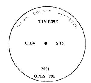
I used a Leica TCA-1100 Total Station and circular prism in the establishment of the new accessories. The Basis of Bearings is the same as that on Minor Partition 1999-025. The distances are to a 5/8"x30" rebar with 1 ½" aluminum cap marked Union county Survey Marker.
