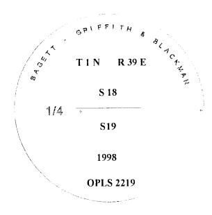
I used a steel tape and magnetic compass in the establishment of the new accessories. I used 18° East declination. Distances are to a 60d spike driven into the root crown of the bearing tree in the right side. A brass washer marked OPLS 2219 was attached to the BT blaze.
