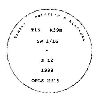
I used a steel tape and magnetic compass in the establishment of new accessories. The magnetic declination used was 17° East. The distance to the bearing trees is to a 50d spike driven on the right side of the tree at the root crown. I attached a brass washer marked OPLS 2219 to the BT blaze.
