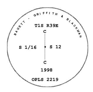
I used a steel tape and magnetic compass in the establishment of new accessories. The magnetic declination used was 17° East. The distance to the bearing trees is to a 50d spike driven on the right side of the tree at the root crown. attached a brass washer marked OPLS 2219 to the BT blaze.
