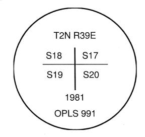
I used a steel tape and magnetic compass in the establishment of the accessories. I used 16° East declination, the distances are to a 60d spike driven into the right side of the root crown of the new bearing trees. In the Northeast bearing tree, the spike is driven in the left hand side. A brass washer marked OPLS 83571 is attached to the BT blaze of the new bearing trees.
