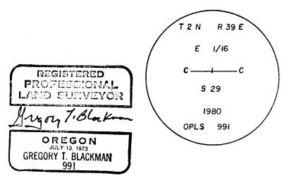
I used a steel tape and a magnetic compass with 20° E declination. I set a brass washer marked OPLS 991 at the BT blaze.
