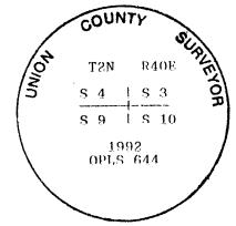
I used a steel tape and magnetic compass in the establishment of new accessories. I used 20° East magnetic declination. The distances are to a 50d spike driven in the right side of the root crown. I attached a brass washer marked OPLS 644 to the BT blaze.
