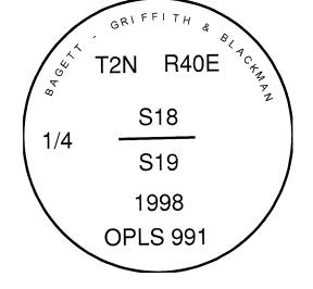
I used a steel tape and magnetic compass in the establishment of the new accessory. I used  $15^\circ$  East declination.
