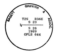
I used a steel tape and magnetic compass in the establishment of new accessories. I used 17° East magnetic declination and the distances are to the chiseled "X" on the bearing object.
