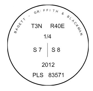
I used a steel tape and magnetic compass in the establishment of the new accessories. I used 16° East declination, the distances are to a 60d spike driven into the right side of the root crown of the new bearing trees. The spike in the Southeast bearing tree is on the left hand side. A brass washer marked OPLS 83571 is attached to the BT blaze of the new bearing trees.
