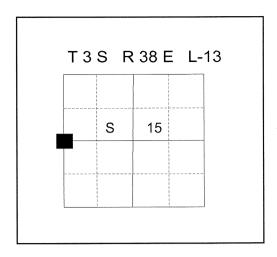
A 5/8"x30" rebar w/ 1½" alum. cap bears N33°W, 14.12 feet, marked UNION COUNTY SURVEYOR NW RP. In 1996, the corner was found and the position documented by GPS observation #9640 by Walter L. Caswell. Monument Record 042-2002R could find no evidence of the corner monument or Northerly references. The Southerly references were found.
