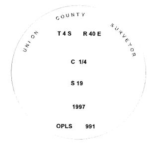
I used a total station instrument in the establishment of the new accessories. I used the same solar observation as survey number 004-1997 as the basis of bearing.
