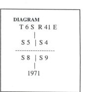
A sawed western larch stump, 17 ins. in diam., bears S. 35° E., 26 1/2 lks. dist., with scribe marks BT visible on open blaze. (Record, 14 lks.)
