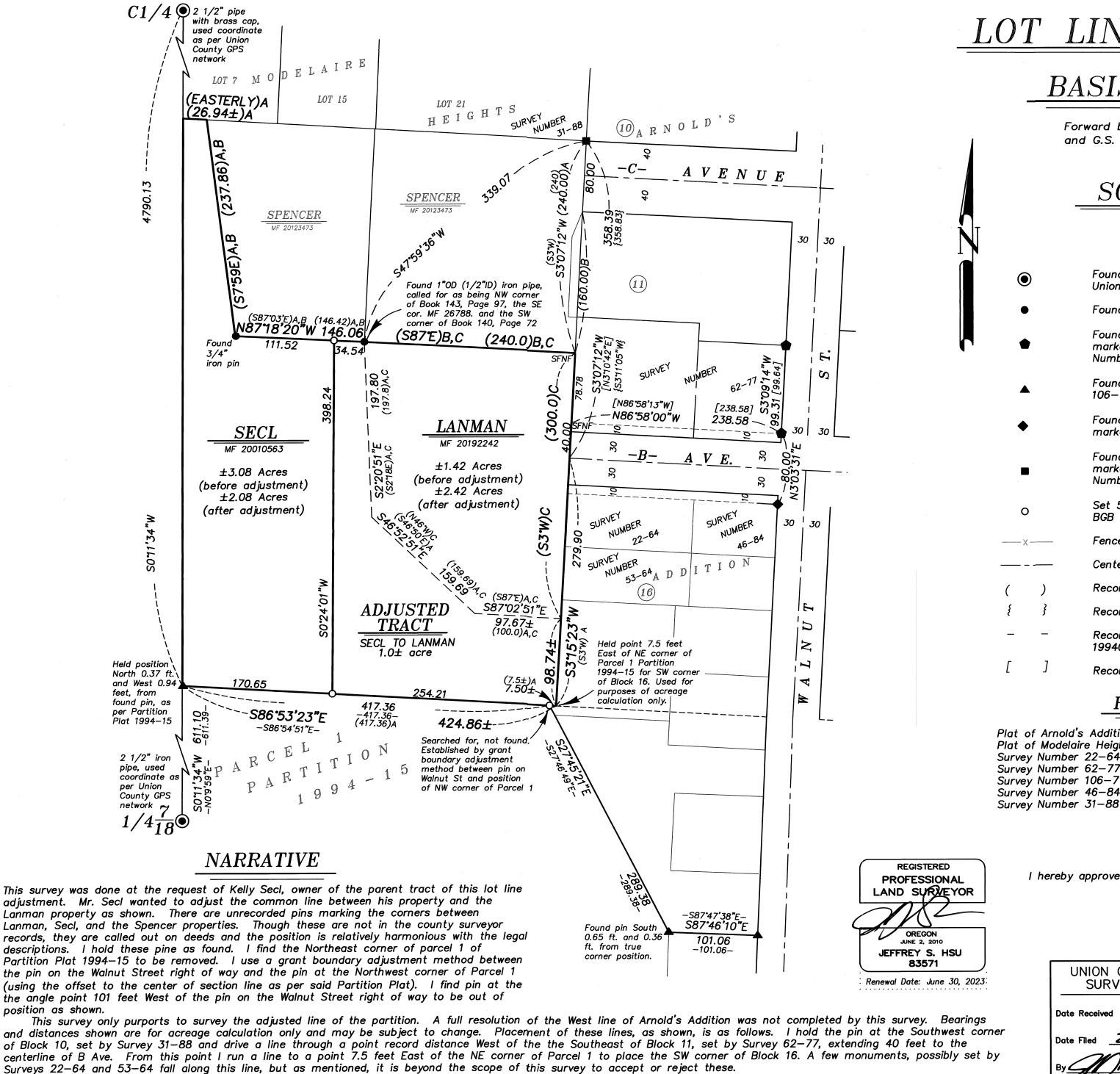
Placement of the line prior to adjustment was done by rotating record deed distances to the found monuments. Angle points do fall in line with lines of possession.
