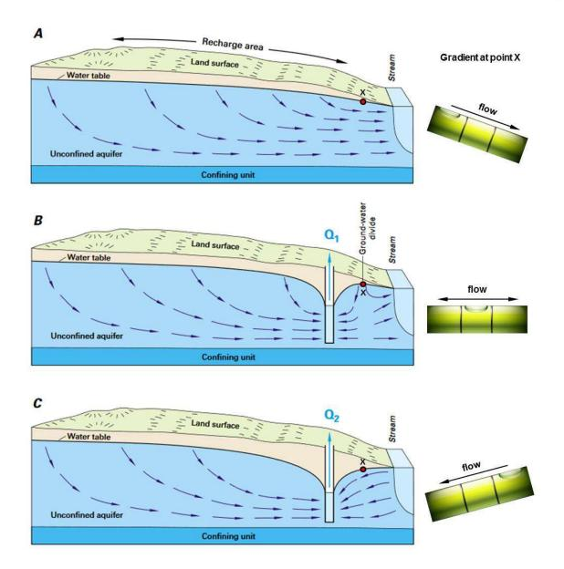
Figure 6. Adapted from Alley, 1999. Diagram showing the development of groundwater capture at two different pumping rates (Q1<Q2) and the impact of pumping rates on hydraulic gradient and ultimately, flow path direction.
