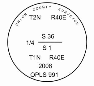
I used a Leica 14 RTK GPS in the establishment of the new accessories. Basis of Bearing is as per Survey 014-2006, the distances are to the center of the aluminum caps of the bearing objects.
