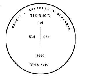
I used a total station with the same basis of bearings as Survey #028-1999 in the establishment of the new accessories. The distances are to the center of the aluminum cap.
