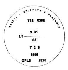
I used a steel tape and magnetic compass in the establishment of the new accessories. I used 18° East declination, the distances are to a 60d spike driven into the right side of the root crown of the bearing tree.
