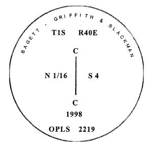
I used a steel tape and magnetic compass in the establishment of the new accessories. I used 18° East declination, the distances are to a 60d spike driven into the root crown of the bearing tree. A brass washer marked OPLS 2219 is attached to the BT blaze.
