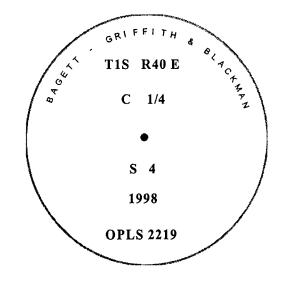
I used a steel tape and magnetic compass in the establishment of the new accessories. I used 18° East declination, the distances are to the center of the caps on the reference pins.
