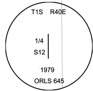
I used a steel tape and magnetic compass in the establishment of the new accessories. I used 14° East declination, the distances are to a 60d spike driven into the right side of the root crown of the bearing trees. A brass washer marked OPLS 83571 is attached to the BT blaze of the new bearing tree. Bearing and distance of the fence post is to the center of post.
