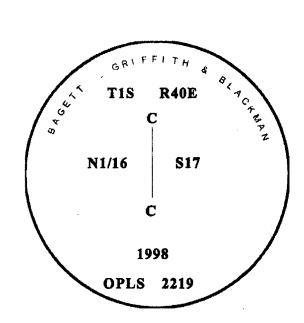
I used a steel tape and magnetic compass in the establishment of the new accessories. I used 18° East declination, the distances are to a 60d spike driven into the root crown of the bearing tree. A brass washer marked OPLS 2219 is attached to the BT blaze:
