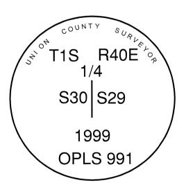
I used a steel tape and magnetic compass in the establishment of the new tree accessory. 16° East declination, the distances are to a 60d spike driven into the right side of the root crown of the new bearing tree. A brass washer marked OPLS 83571 is attached to the BT blaze of the new bearing trees. Bearing and distances to the iron pin accessory were determined by GPS observation with a Leica GS-15 unit. The Basis of Bearing is as per Survey Number 013-2015.
