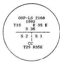
I used a steel tape and magnetic compass in the establishment of new accessories. I used 20° East magnetic declination.
