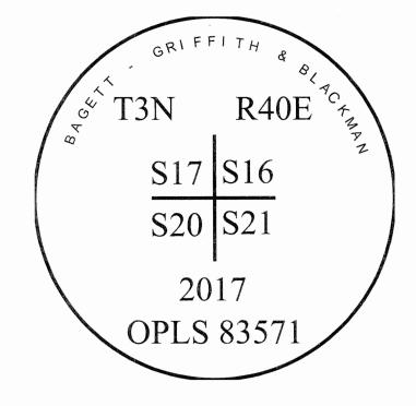
I used a steel tape and magnetic compass in the establishment of the bearing trees and objects. Magnetic declination used was 13° East. Bearing is to a brass washer marked OPLS 83571 in the lower blaze of the trees. Distance is to a spike set in the root crown of the side of the trees.
