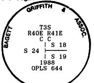
OREGON JULY 10, 1964 **DUANE I. GRIFFITH**  I used a steel tape and magnetic compass in the establishment of new accessories. I used 18° East magnetic declination and the distances are to a 50d spike driven in the right side of the root crown. I attached a brass washer marked OPLS 644 to the BT blaze.
