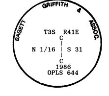
I used a steel tape and magnetic compass in the relocation of the existing accessories. I used 20° magnetic declination. The distances are to a 50d spike driven in the right side of the root crown.
