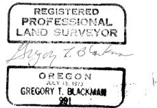
I used a steel tape and magnetic compass in the establishment of new accessories. I used 20° East magnetic declination and the distances are to a 50d spike driven in the right side of the root crown. I attached a brass washer marked OPLS 991 to the BT blaze.
